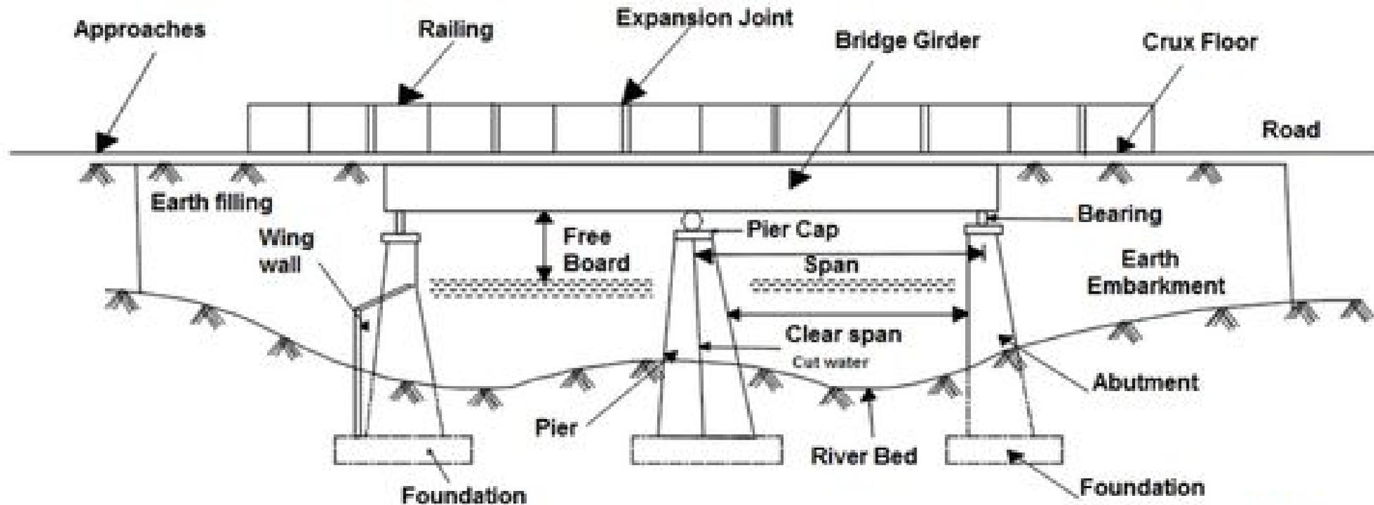
**Component Parts of the Bridge structure**
