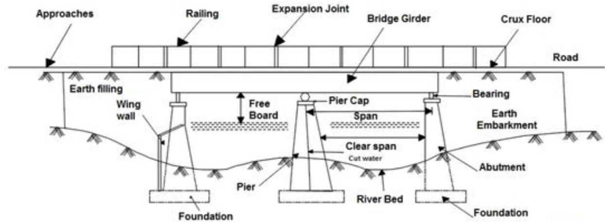
**Component Parts of the Bridge structure**
